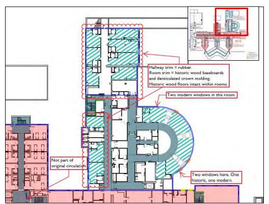
*Figure 20:* Third Floor, Maternity Ward – Showing Location of Intact Original/Historic Features Including Wood Floors, Wood Base Trim, Wood Chair Rail, and Denticulated Crown Molding (CPG, 2023)
