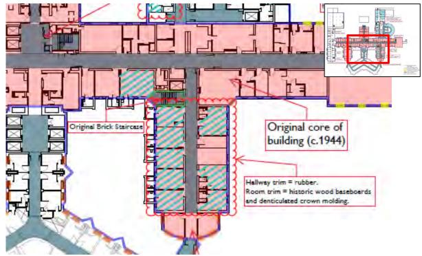
*Figure 11:* Third Floor, Front Southeast Wing of Original c.1944 Section – Showing Location of Intact Original/Historic Features Including Wood Floors, Wood Base Trim, Wood Chair Rail, and Denticulated Crown Molding (CPG, 2023)
