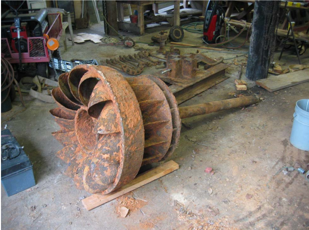
Mill Turbine During 2010 Refurbishing Project
