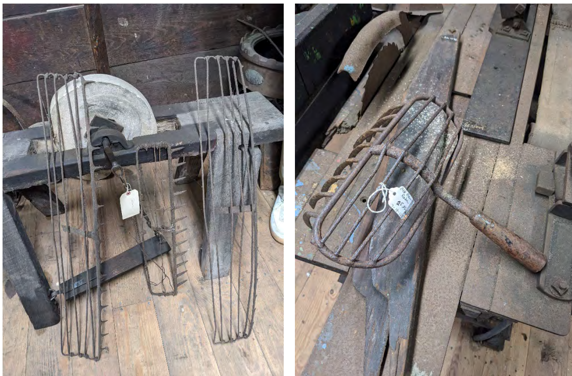
Figure 1: Metal components of oyster rakes (left) and a clam rake (right) that remain in the Samuel D. Outlaw Blacksmith Shop, September 2022. Courtesy of the Virginia Department of Historic Resources.
