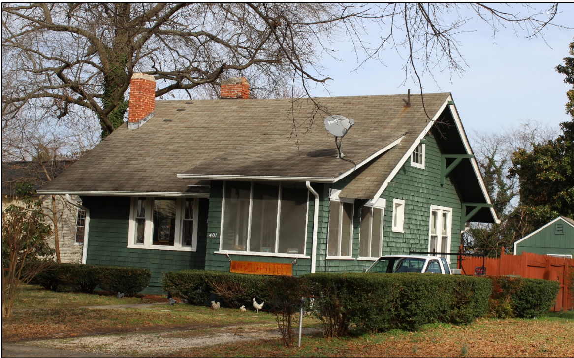
Figure 18. “The Loraine” in “A Village” at 401 Spruance Street (116-5160). Beneath the screened porch, the side-entry door and the smaller rectangular front window match the plan. March 2019.
